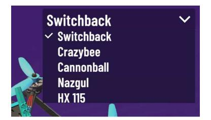
The selection of models falls into different model classes: Switchback: 5inch racing quad Crazybee: Micro quad Cannonball: Mega quad (10inch props) Nazgul: 5inch Freestyle HX 115: Toothpick (2.5inch props)
